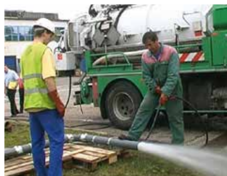
The S and Plus ranges, assembled and anchored, have successfully passed a high-pressure jetting test: cleaning pressure of 120 bar from the pump, which means 100 bar at the nozzle outlet, without leaks or misalignment.
