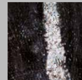
Zinc coated: a white line of zinc salt shows that the damage is completely plugged
