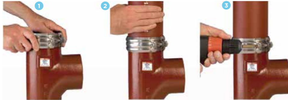
1 - Push the supplied assembled coupling onto the pipe spigot so that it abuts on the central register of the elastomer gasket.
